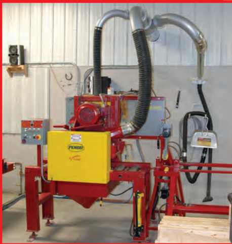
Inline Top Edge Planer & Dust/Chip Collector
